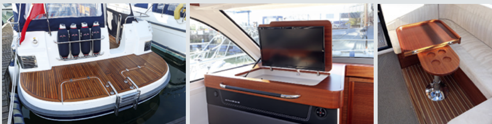
1. Scandinavians like big bathing platforms and fender storage. 2. A TV sits inside the chart table. 3. The joinery throughout this craft is superb.
